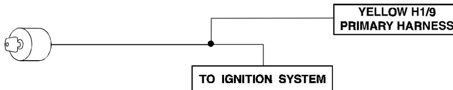
**H1/10 BROWN** (+) siren output: Connect this to the red wire of the 514T Revenger™ siren. Connect the black wire of the siren to (-) chassis ground, preferably at the same point you grounded the control module's H1/8 BLACK wire.
