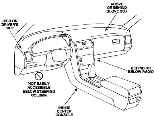
The higher the control module is in the vehicle, the better the transmitter range will be. If you put the control module under a seat or inside a metal dashboard, range will suffer, and you may wish to add a 542T Range Extending Antenna (available separately).
