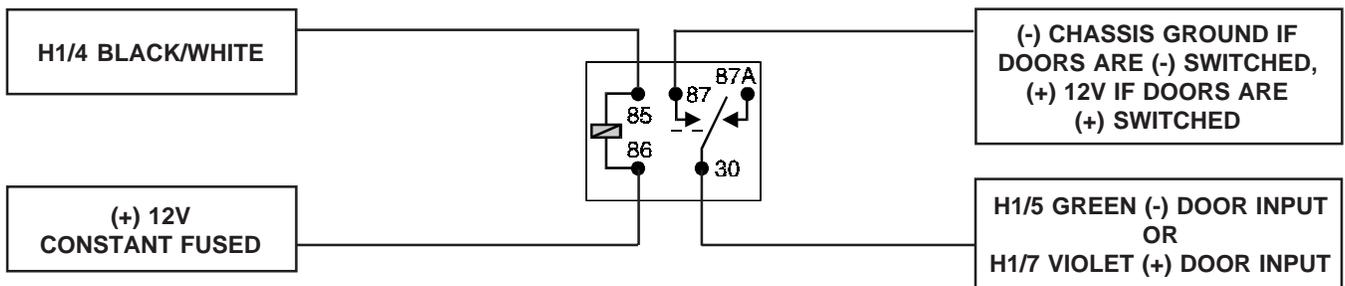
**H1/5 GREEN** (-) door trigger or **H1/7 VIOLET** (+) door trigger input: If the door switch wire you found is (-) when the door is open, connect the GREEN wire to it. If the door switch wire you found is (+) when the door is open, use the VIOLET wire instead.
