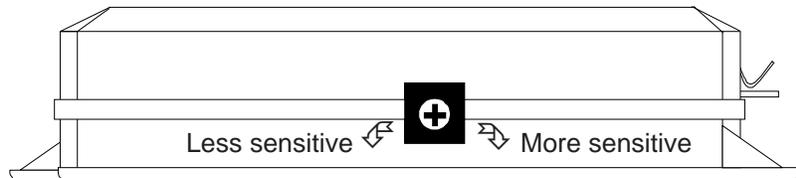
There is a full-fledged Stinger™ shock sensor inside the control unit. Adjustments are made via the rotary control as indicated above. Since the Stinger™ shock sensor does not work well when mounted too firmly to metal, we recommend *against* screwing down the control module.
