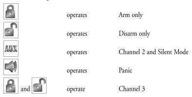
The expanded configuration also allows the user to utilize Multi-Level Security Arming, a feature that cannot be accessed from a standard configuration transmitter.
