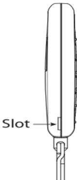
1. Using a small flat-headed screwdriver, insert into slot located on the side of the remote control and carefully pry open the unit.
