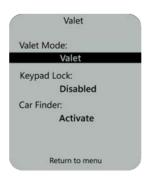
When Valet is selected, press **FUNCTION** to save and transmit the command. When the command is received at the vehicle, a confirmation tone will play, and the cursor will exit the feature. The Valet text will now be displayed to identify the current system status. If the command fails to execute at the vehicle, the text will revert to OFF and error tone will play.
