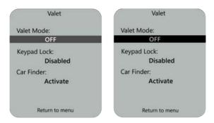
With the feature selected, **LOCK** and **UNLOCK** will cycle through the available options for that feature (Valet/OFF).
