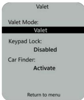
When Valet is selected, press **FUNCTION** to save and transmit the command. When the command is received at the vehicle, a confirmation tone will play, and the cursor will exit the feature. The Valet text will now be displayed to identify the current system status. If the command fails to execute at the vehicle, the text will revert to OFF and error tone will play.
