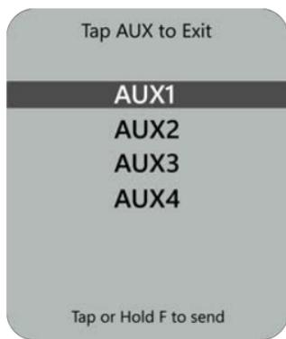
**LOCK** and **UNLOCK** are used to navigate up and down through available AUX outputs. When the intended AUX is highlighted, press **FUNCTION** to activate the output. For extended AUX commands (validity) continue holding the **FUNCTION** button for the desired duration.
