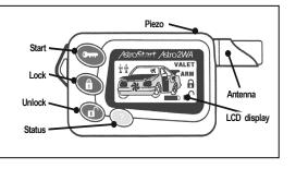
When used with a **4204**, immediately after a command is sent, the remote control switches to receive mode for 5 seconds while waiting for a confirmation signal. The only exception is for the Start command. The remote will always stay in receive mode, waiting for engine shut down feed back from the car.
