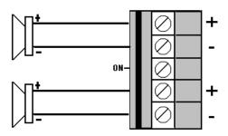
**NOTE:** The dual + and – subout terminals of the d2500.1 are paralleled internally and the combined load impedance should be taken into consideration when connecting multiple subwoofers.
