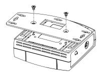
Mounting TOY-SC1 with SIRIUS SCC1 Bracket Assembly
