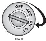
To disarm the security system, turn the ignition key on and press and release the Valet switch within 15 seconds. The
