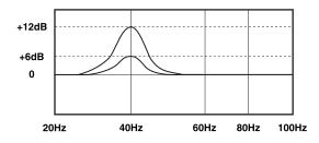
**CAUTION!** *QBASS™* should only be used in systems with strong subwoofers. 12dB is a lot of bass boost and could damage full range speakers.
