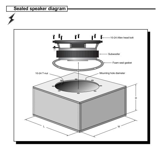
Internal dimensions should be calculated to determine the correct box volume. Be sure to allow for speaker displacement and extra bracing (if used).
