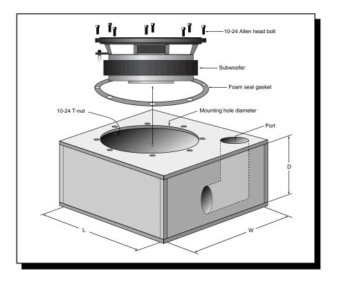
Internal dimensions should be calculated to determine the correct box volume. Be sure to allow for speaker displacement, extra bracing (if used), and port displacement. It may be necessary to angle the port to fit your design. To calculate volume of the port: Radius<sup>2</sup> x 3.14 x Length of port.
