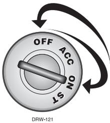
Turn ignition to "on" position, turn to "off" position. Press and release the integrated LED/Valet® switch within 10 seconds. The status LED will
