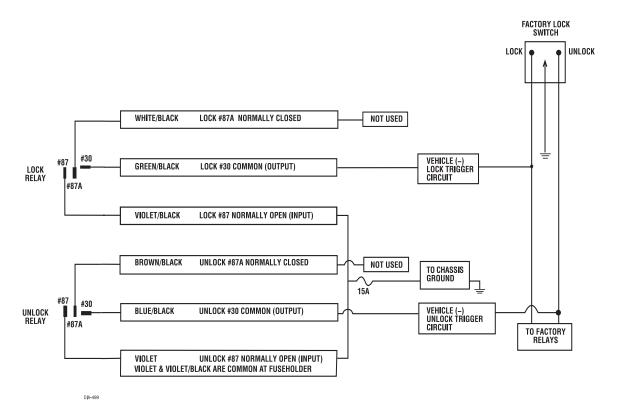
Wiring Diagram C, Directly-Wired Reversing-Polarity Switch Circuits
