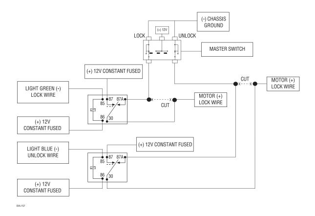
**IMPORTANT!** If these are not connected properly, you will send (+)12 volts directly to (-) ground, possibly damaging the alarm or the factory switch.
