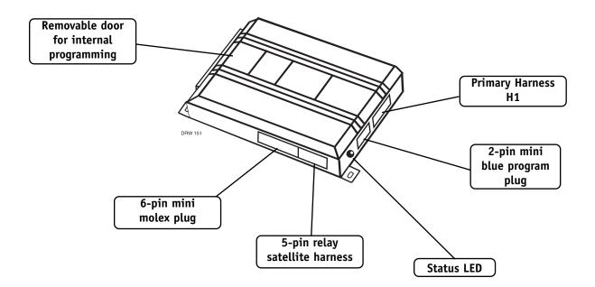
\*NOTE: When installing this system, be sure to plug the 542G range-extender antenna into the white 2-pin plug of the control module.
