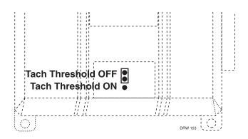
In most cases, this jumper can be left in the OFF position. Some new vehicles use less than 12 volts in their ignition systems. The unit may have trouble learning the tach signal in these vehicles. Changing the jumper to the ON setting changes the trigger threshold of the digital tach circuit so it will work properly with these vehicles. The vehicles affected include many newer Dodge/Chrysler/Plymouth vehicles, such as the Neon, Cirrus, Stratus, Breeze and LH-based vehicles.
