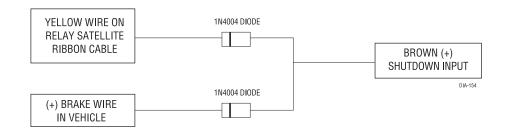
**IMPORTANT!** Once the interface is complete, attempt to remote start the vehicle with the door closed and the key in the ignition. The vehicle should not start. If it does, re-check the connections.
