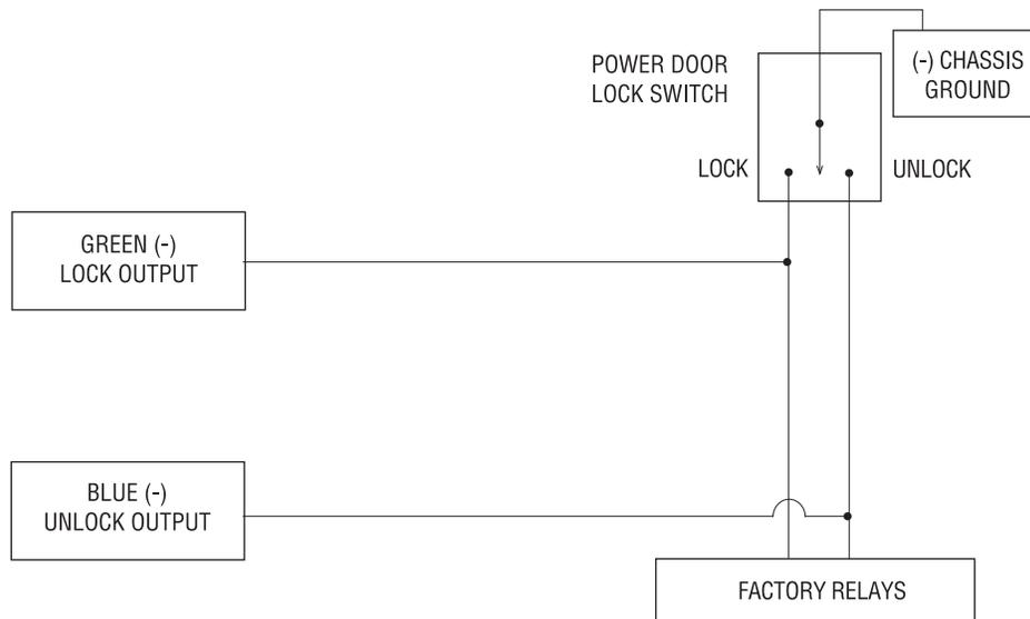
**IMPORTANT!** Remember that the functions of these wires reverse between Type A and Type B!
