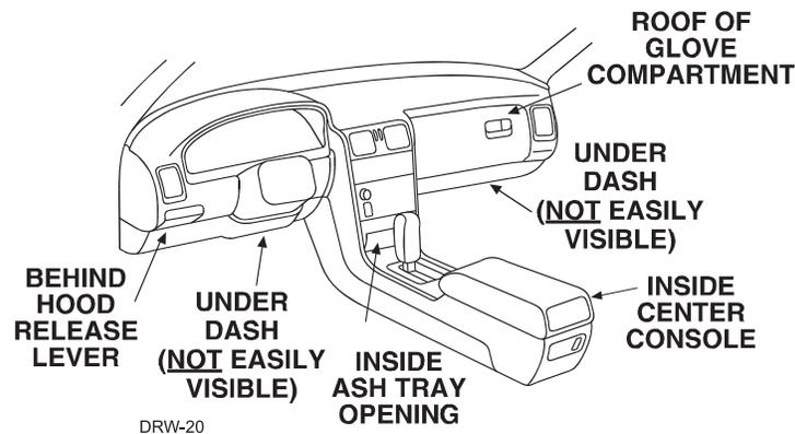
This system has Remote Valet. The user can enter and exit Valet® Mode without having to reach the Valet/Program switch. This feature was introduced so that switch location was less critical in day-to-day use. As long as the Valet/Program switch can be reached to disarm without a transmitter, easy access is not important.
