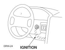
5. Now turn the key to the start position. The meter display should stay steady, not dropping by more than a few tenths of a volt. If it drops close to or all the way to zero, go back to Step 3. If it stays steady at (+)12V, you have found an ignition wire.
