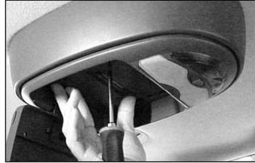
7. The trim panel should be flush to the headliner without gaps. If any gaps occur, adjust the length of the spacers and/or cut the trim panel to the correct shape.
