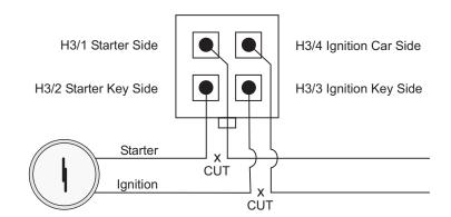
**NOTE:** The diagram below shows the module side of the connector (looking into the female pins).
