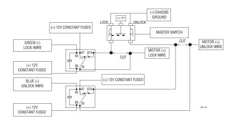
IMPORTANT! Do not connect the outputs of the alarm directly to the actuator.
