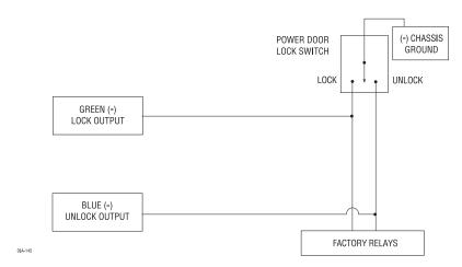
**IMPORTANT!** Remember that these wires' functions reverse between Type A and Type B.
