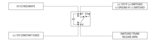
**IMPORTANT!** Never use this wire to drive anything except a relay or low-current input! The transistorized output can only supply 200 mA of current. Connecting directly to a solenoid, motor, or other high-current device will cause it to fail.
