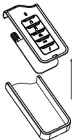
2. Turn both the unit front and circuit board over, remove battery from clip and replace.
