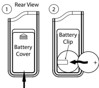
1. Slide the battery cover up by applying equal pressure at its top and bottom (the arrow on the cover indicates the direction), remove the cover from the remote control housing.
