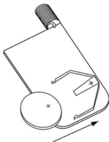
**Note** Verify that the battery polarity is correct when replacing.
