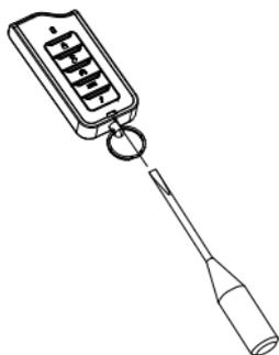
1. Using a small flat-head screwdriver, insert into slot located at the bottom of the keypad and carefully pry the front of the unit open.
