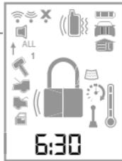
The alarm arms, doors lock (if connected), and the siren chirps and parking lights flash once. The **ARMED** text and beeps play to confirm and the System Status Icons update. If Valet mode\* is On, the doors lock and the **VALET** text and tone play. Exit Valet mode to arm the alarm normally.
