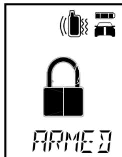
**Details:** The siren in the vehicle will “chirp” once and the parking lights will flash once. If the power door locks have been connected, the doors will lock. The system will automatically check for errors when it arms. The 2-way remote will “chirp” once and the lock icon appear to confirm arming. If no arm confirmation is received, the remote will give the Out-Of-Range signal.
