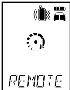
minutes and 1 minute of runtime remaining, it sends the 2-way remote control a paging signal.
