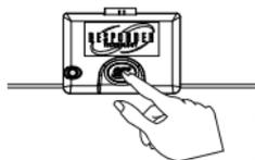
At anytime during the next 10 seconds, press and release the Valet switch. Now the Status LED lights constantly if you have entered Valet® Mode, and shuts off when exiting Valet Mode.
