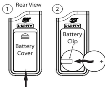
1. Slide the battery cover up by applying equal pressure at its top and bottom (the arrow on the cover indicates the direction), remove the cover from the remote control housing.
