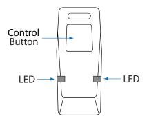
The Control Center, typically located on the upper part of the front windshield. It consists of:
