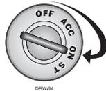
To disarm the system, turn the ignition key on and press the Valet switch within 15 seconds.
