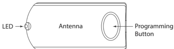
The Antenna, typically located on the upper part of the front wind-shield, sends and receives commands or messages to and from the system. It consists of:
