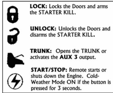
Pressing the Lock and UNLOCK buttons simultaneously will activate the Aux 2 output.
