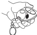
**4. Program the feature:** While holding the integrated LED/Valet® switch, assign the selected feature to the factory keyless transmitter button by either pressing Lock for a 1 chirp setting or pressing Unlock for a 2 chirp setting.
