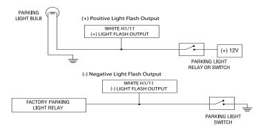
**Note:** For parking light circuits that draw 10-amps or more, the internal jumper must be switched to a (-) light flash output. (See Setting the light flash polarity section of this guide.) P/N 8617 or a standard automotive SPDT relay must be used on the H1/11 light flash output harness wire.
