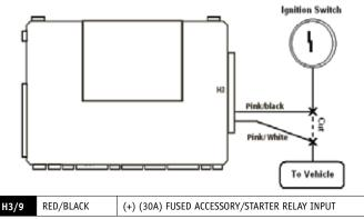
This wire is the polarity feed to the accessory and starter relays.
