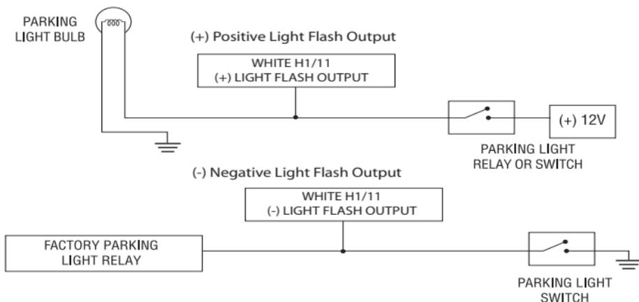
**Note:** For parking light circuits that draw 10-amps or more, the internal jumper must be switched to a (-) light flash output. (See Setting the light flash polarity section of this guide.) P/N 8617 or a standard automotive SPDT relay must be used on the H1/11 light flash output harness wire.
