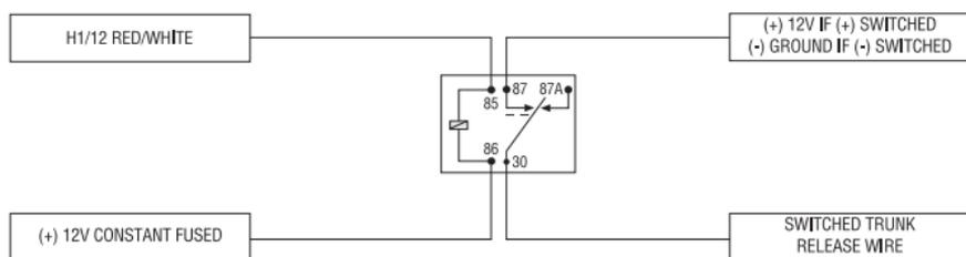
**Warning!** Never use this wire to drive anything but a relay or a low-current input, supplied output is only 200mA. Connecting directly to a solenoid, motor, or other high-current device will cause the module to fail.
