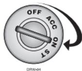
1. Insert the key. Turn the ignition to the ON position. The heavy gauge pink wire must be connected.
