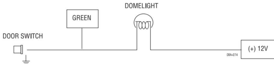
\*Door trigger input is needed if one of the following are used: MTS, passive arming, auto re-locking, door ajar error honk or Smart Key control.
