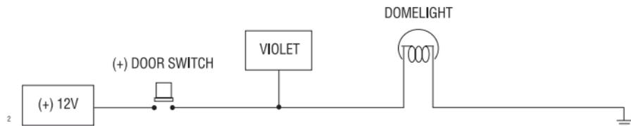
\*Door trigger input is needed if one of the following are used: MTS, passive arming, auto re-locking, door ajar error honk or Smart Key control.
