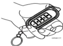
3. Transmit. Press the
